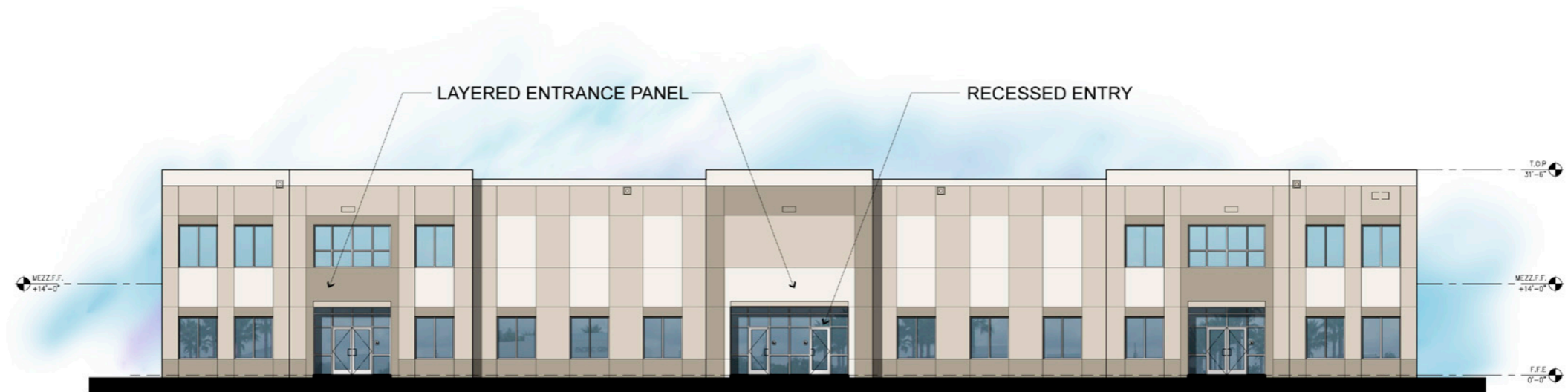
BUILDING 3-EAST EXTERIOR ELEVATION SCALE: 1/8"=1'-0" (A)
